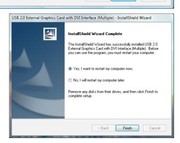
9. If installing more than one converter, select "No, I will restart my computer later" and click "Finish" to continue with the installation of the second converter. Connect the next display device to the
